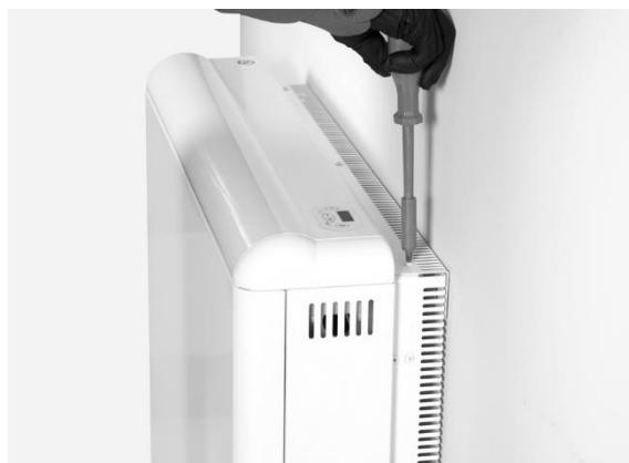
**ECO ARC MUST NOT BE HUNG ON THE SCREWS;** these are used only to prevent the device from overturning and not to support it. If there is any doubt concerning the wall strength, consult the corresponding construction specialist. The appliances are heavy; it is the installer responsibility the correct installation and wall support of these devices to prevent them from overturning.
